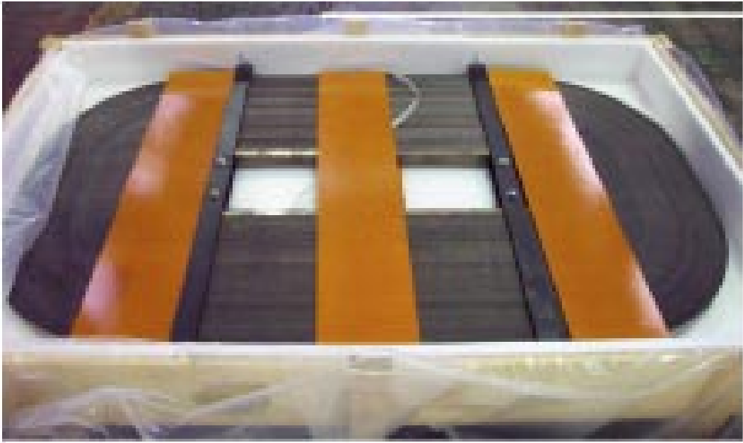
Fig. 4 MA core for rf cavity.
