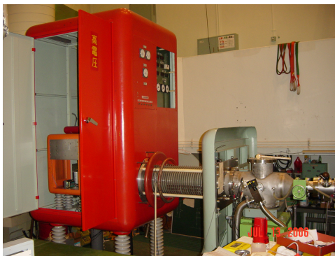
Fig. Cockcroft-Walton type Accelerator and Tritium Target
