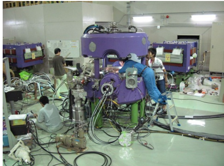
2. Repair and commissioning of Injector cyclotron (Sep - Dec 2008)
