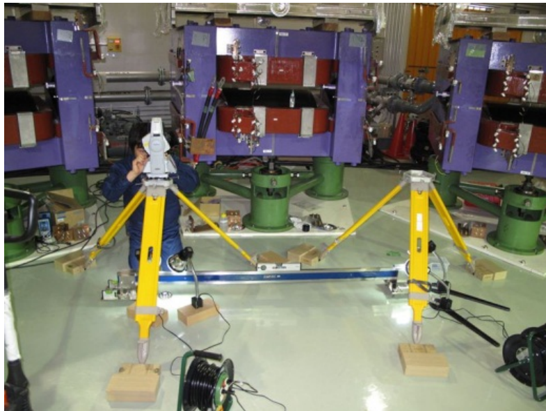
3. Setting up Monuments for Alignment (Mar – May 2009)
