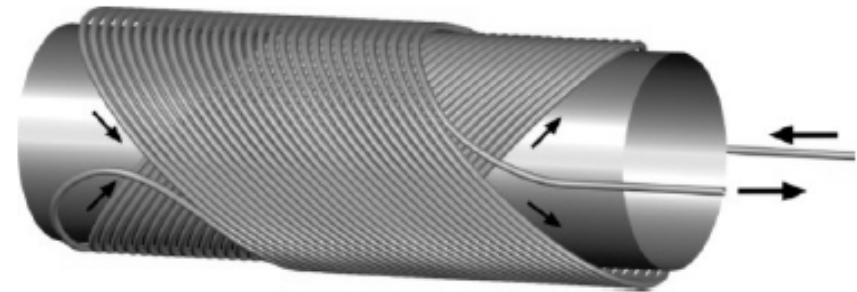
Figure 2. Example of a 2-layer winding used to form a DH dipole magnet
