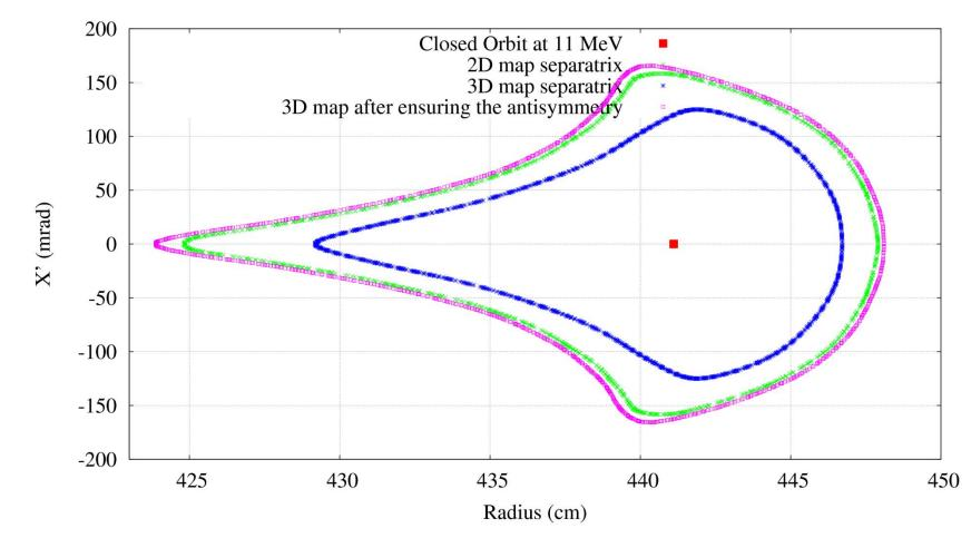
The previous problem seem to arise from the Bx, By components that introduce some discontinuities in the calculation of the field and its derivatives in the median plane of the FFAG. Is the median plane antisymmetry guaranteed in real life?
