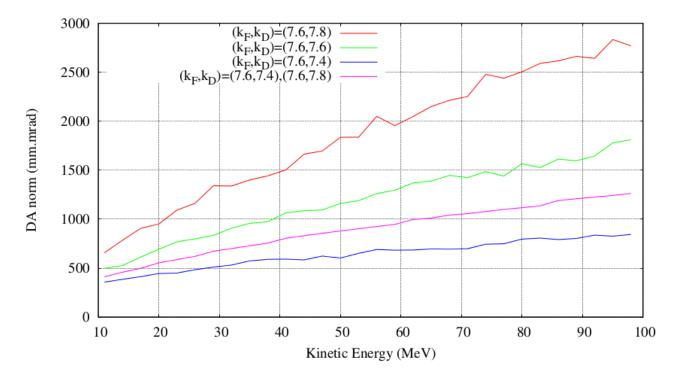
Increasing kD generally increeases the Dynamic Acceptance. Therefore alternating the differences of kF,kD in order to fix the tune has a smaller DA than the equivalent scaling FFAG case.
