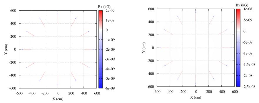
Field map plot of the Bx and By component in the median plane of the 150 MeV KURRI FFAG. If the median plane antisymmetry were ensured, one would ontain a blank map (zero everywhere). Antisymmetry not ensured.
