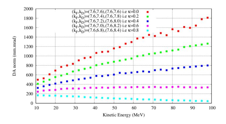
Increasing the differences of the scaling factors differences i.e.  $\kappa = k_D - k_F$  decreases the DA of the machine.
