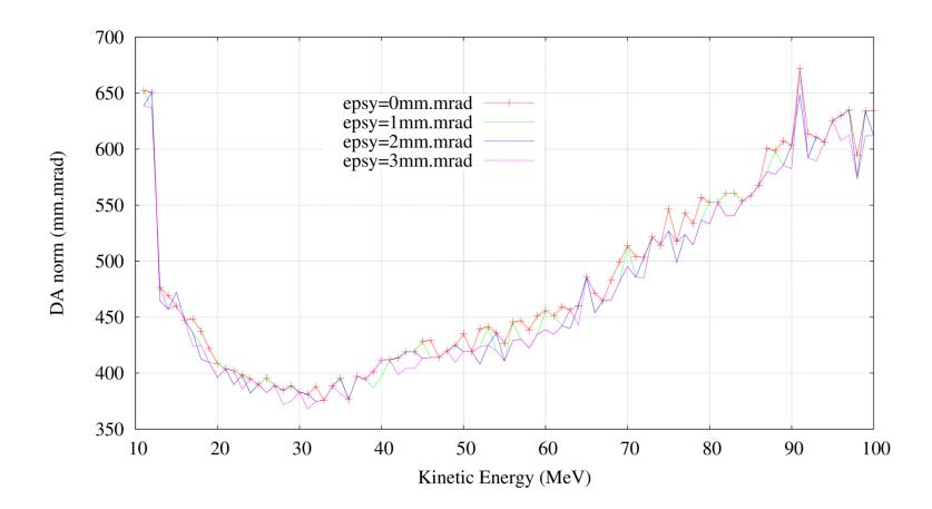
The Dynamic Acceptance is around 375 mm.mrad and seems insensitive to the vertical amplitude Vertical amplitude limited to +-1cm, i.e. 3 mm.mrad
