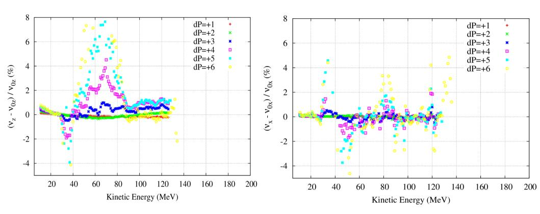
A relative error of less than 8% is obtained in both planes with small increments in P (dP less than 6 mrad)
