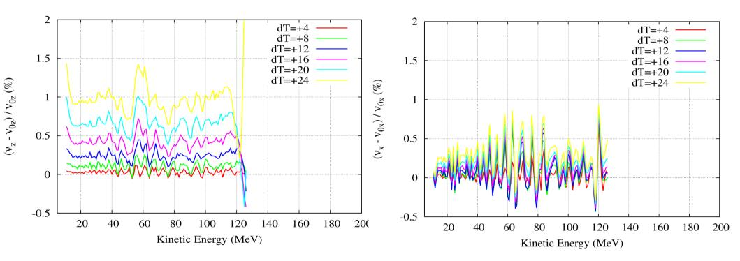
A relative error of less than 1.5% is achieved in both planes with small increments in R (dR less than 1cm)
