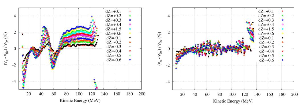
A relative error of less than 4% is obtained in both planes with small increments in Z (dZ less than 0.6 cm)
