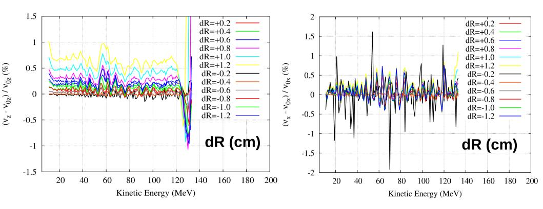
A relative error of less than 1.5% is achieved in both planes with small increments in R (dR less than 1cm)
